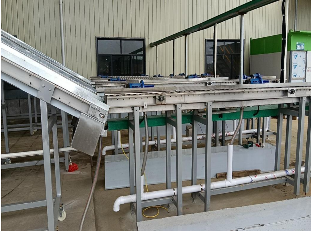
Automatic electrolyte discharging machining for used lead acid batteries
