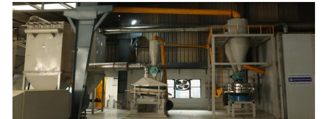
Battery breaking, black mass production, Al/Cu fractions, polypropylene
